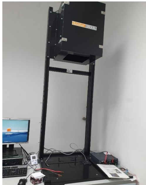
Figure 2.17. The QuickSun 120CA-XL flash solar simulator system used for I-V measurements in the GÜNAM research center.
