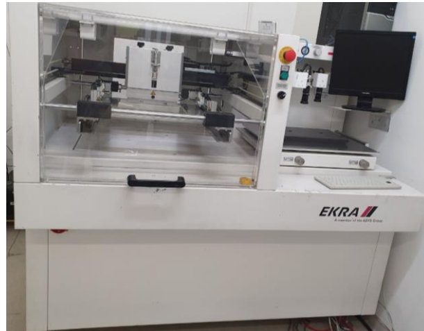
Figure 2.6. Screen printer system in GÜNAM research center.
