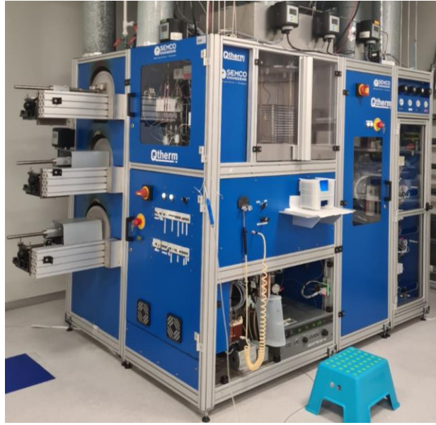
Figure 2.2. SEMCO LYDOPTM furnace (PECVD system) in GÜNAM research center.
