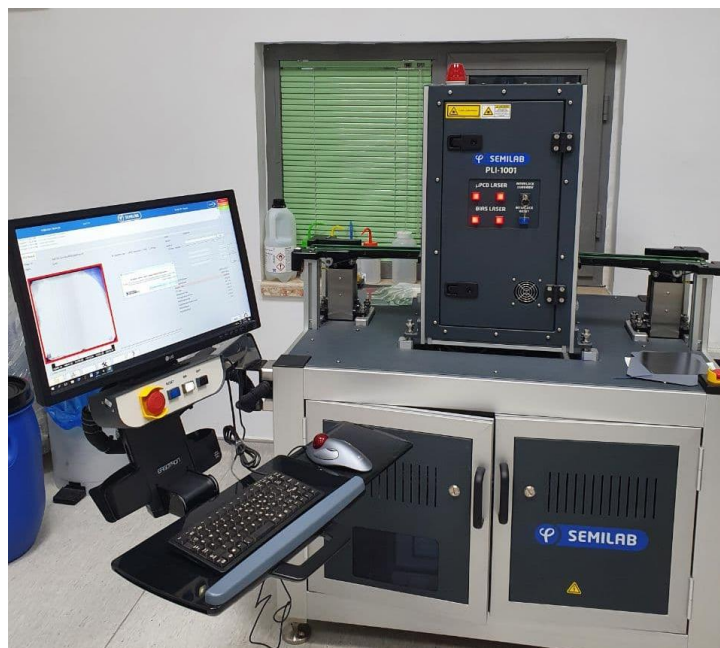
Figure 2.16. Photoluminescence Inspection System in GÜNAM research center.
